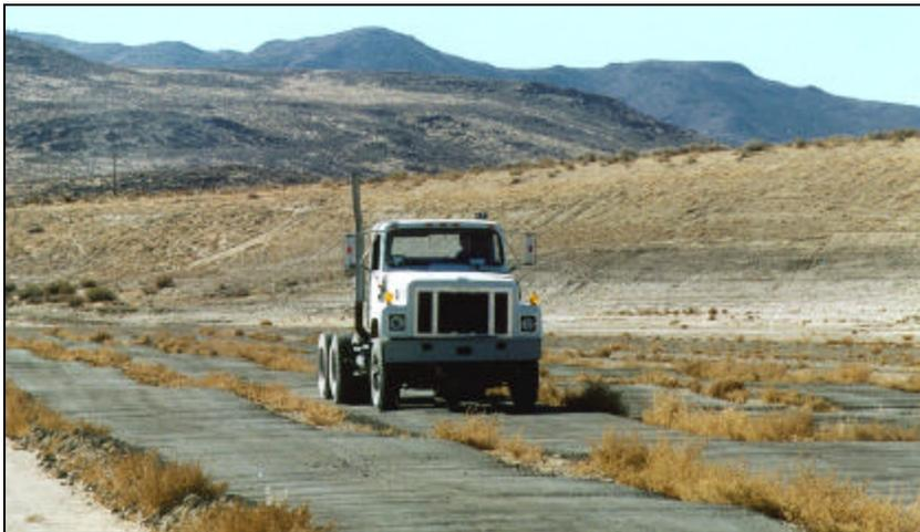
NATC also has dedicated ride quality (RMS) and shock and vibration test courses that are meticulously profiled to quantify shock and vibration inputs. Our road profiling methodology using the Dynamic Force Measurement Vehicle allows us to create test course
